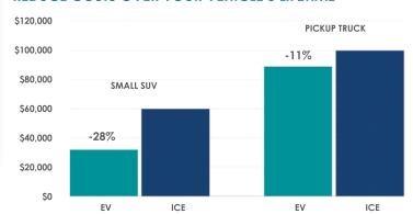
Comparison of an electric vehicle (EV) model to a comparable internal combustion engine (ICE) in a rural environment. Total cost of ownership includes purchase costs, fuel costs, maintenance costs, and insurance costs.
